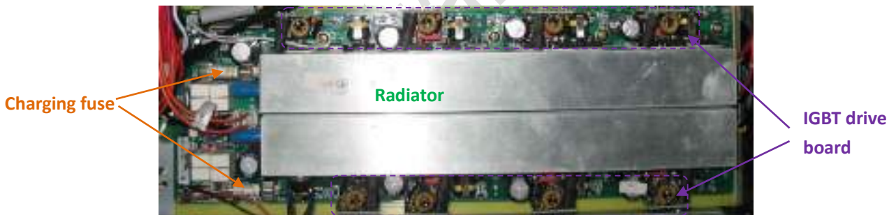
Figure24.PFC power board (15-20K)
