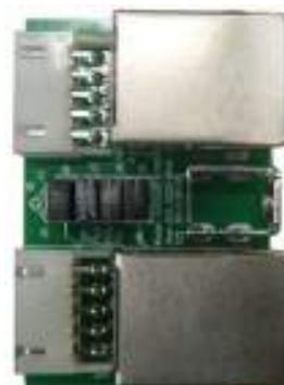
Figure 22. RJ45 interface board interface
