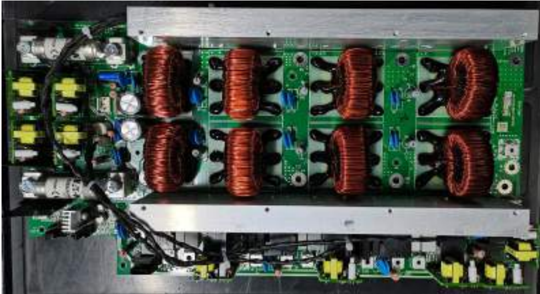
Figure 12. PFC inductor board
