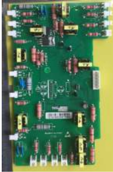
Figure 13.PFC drive board interface
