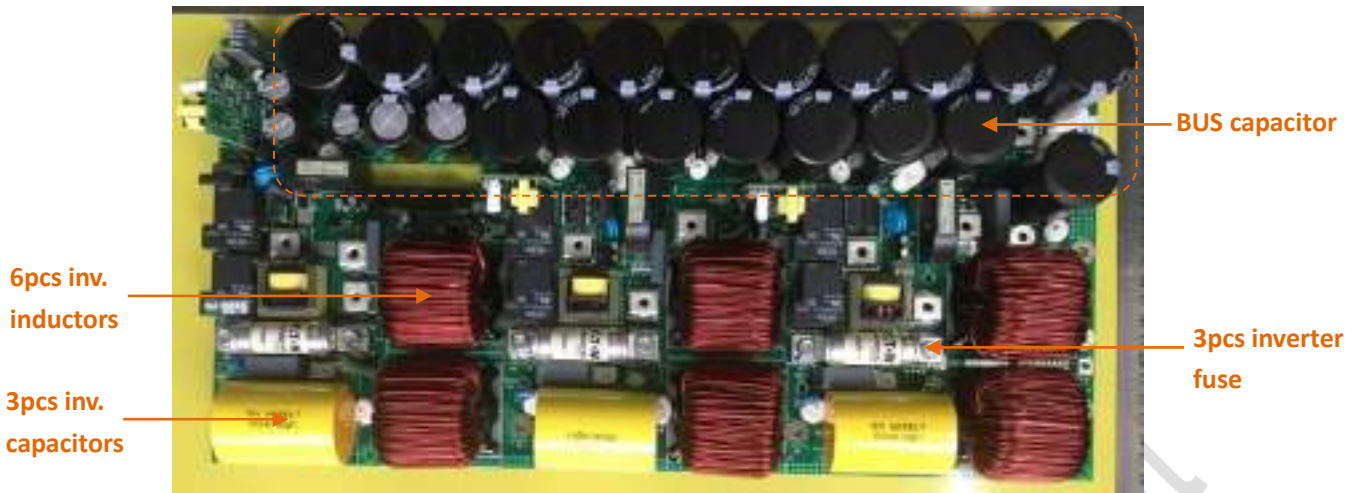
Figure20. Inverter inductor board (40K)
