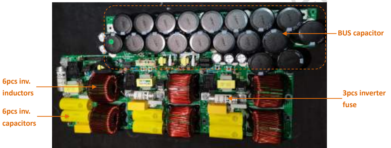
Figure18. Inverter inductor board (15-20K)
