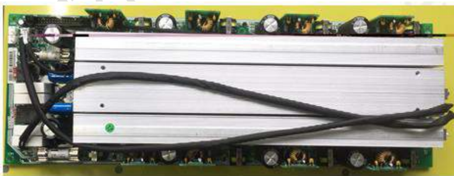
Figure 14 PFC power board
