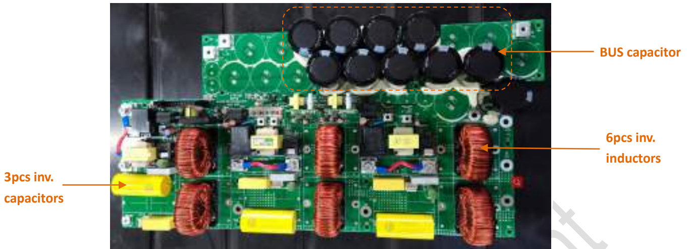
Figure17. Inverter inductor board (10K)
